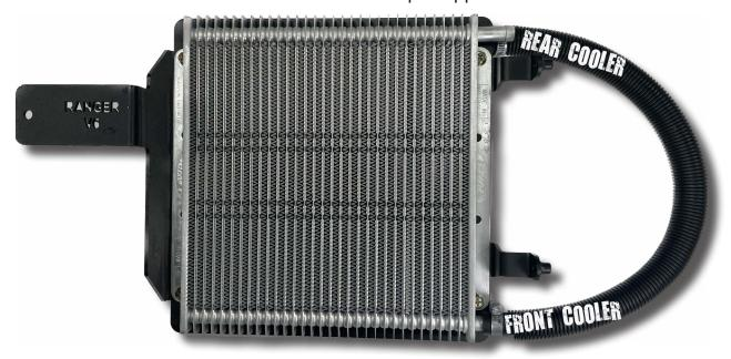
Coolers are omni-directional, so the direction of flow is not important. However for maximum efficiency and effectiveness we recommend the hot oil enters the rear cooler first.
