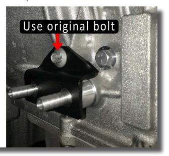
1.28. Route cooler lines to the unions and trim to the correct length. Secure using the hose clamps provided. For the best cooling performance we recommend the hottest oil (from the rear union) goes through the rear cooler first. Ensure that hoses are secure away from moving parts with no kinks that may impede flow.
