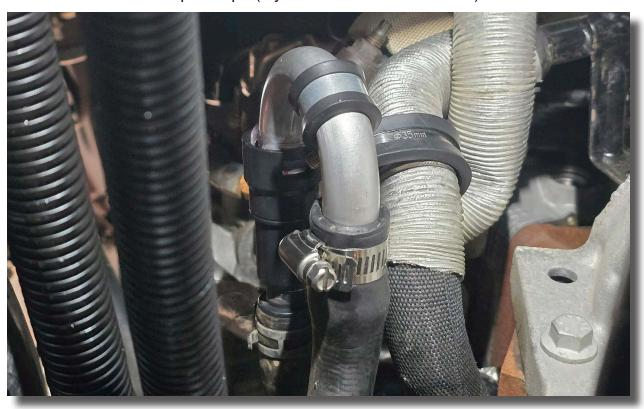
1.27. Install the supplied custom cooler unions. Check that each union has two (2) o-rings fitted prior to installation, and apply a small amount of transmission fluid to both o-rings on both unions to provide lubrication. Install the unions by carefully inserting them into the empty fittings in the side of the transmission left behind by the removal of the heat exchanger. Secure the new unions with the supplied bracket, using one of the T40 Torx bolts previously removed from the heat exchanger.
