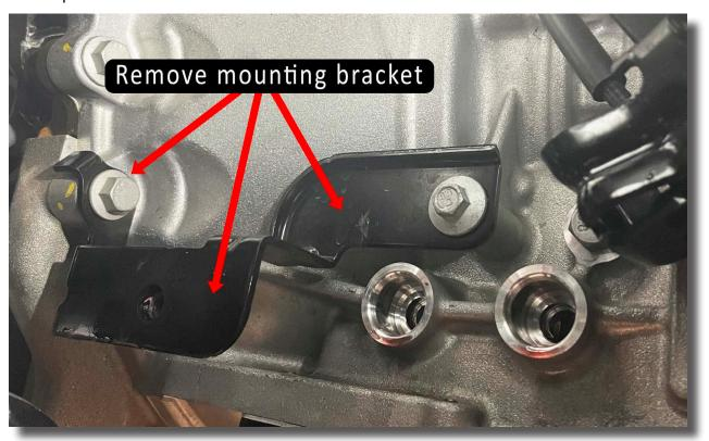
1.25. Reconnect the gear shift cable bracket using the two (2) M10 washers as spacers where the heat exchange bracket was removed.
