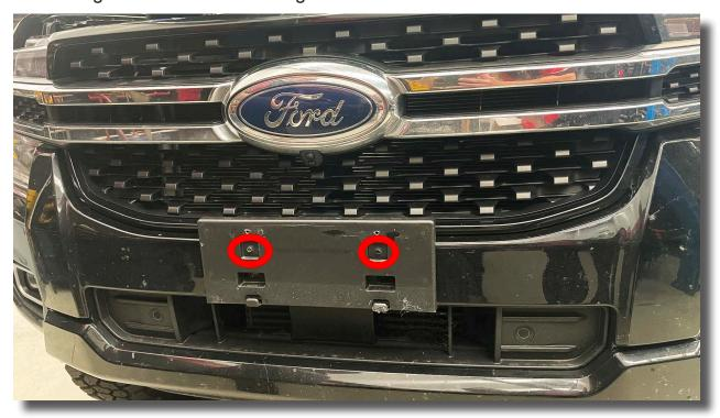
Working along the base of the grill, pull forward to dislodge the clips holding it in 1.8. place. Clips can be difficult to dislodge and may need to be released from behind the grill
