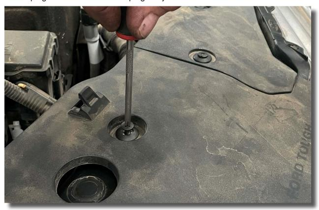
Using a T30 Torx bit, remove the screw holding the air inlet snorkel to allow you to 1.4. easily remove and reinstall the radiator cover.
